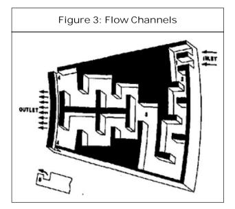
for more than one velocity head of pressure drop. This large number of stages is packaged into a radial wall as small as 11/8 inches (28 mm). Therefore a pressure drop of 3000 to 4000 psi (200 to 300 kg/cm<sup>2</sup>) is achieved by each channel in a very tight space.
