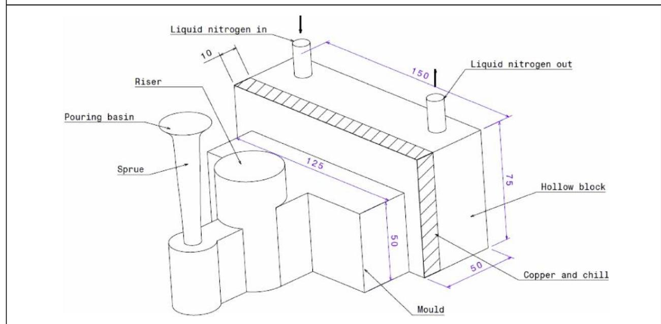
Figure 2: Copper End Chill in a Steel Hollow Block (Brazed) for Passing Liquid Nitrogen
