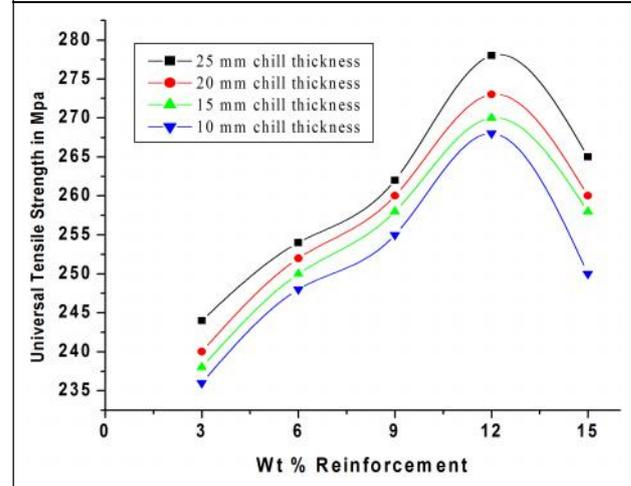
12 wt. % using 25 mm copper end chill thickness invariably has the highest tensile strength.
