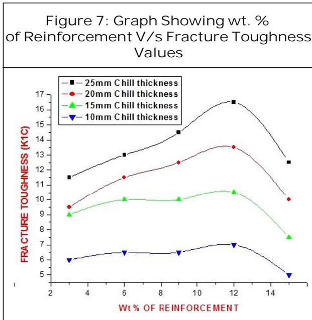
toughness. Further it is observed that fracture toughness value decreases when 15 wt. % reinforcement were present.
