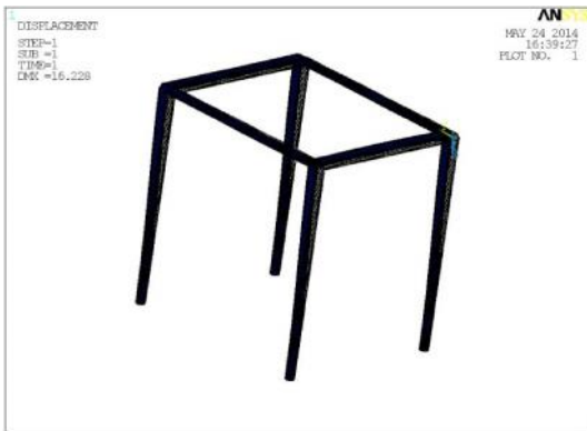
Figure 17: Displacement in Hollow Circular Cross Section When Subjected to Rear Loading
