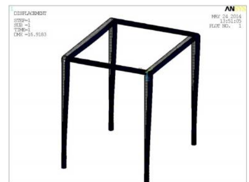
Figure 15: Displacement in Circular Cross Section When Subjected to Side Loading
