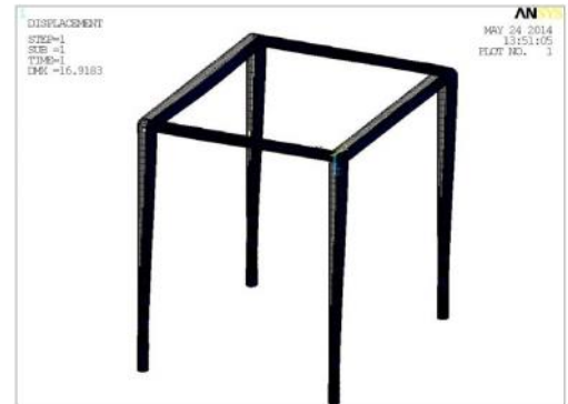
Figure 15: Displacement in Circular Cross Section When Subjected to Side Loading
