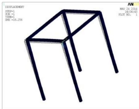
Figure 29: Displacement in Hollow Square Cross Section When Subjected to Rear Loading
