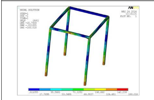
Figure 23: Displacements in Square Cross Section When Subjected to Rear Loading
