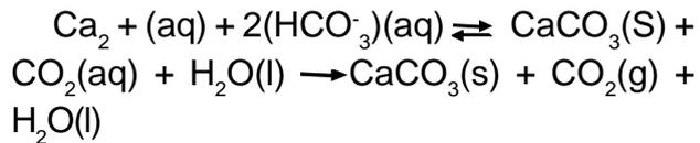
The resulting calcium carbonate  $\text{CaCO}_3$  (Calcite polymorph) is heat-insulating and is therefore is effected for the heat transfer in a heating element. The above reaction is actually a compilation of two equilibrium reactions.
