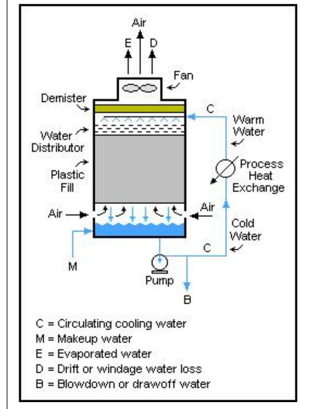
in power plants, petroleum refineries, petrochemical plants, natural gas processing plants, food processing plants, semiconductor plants, and other industrial facilities. A cooling system consists of a cooling unit (e.g., cooling tower) and a heat exchanger in Figure below. Cool water is pumped from the cooling tower and circulated through a heat exchanger to remove heat (i.e., to cool) from hot process fluids generated in HVAC or other industrial process equipment.
