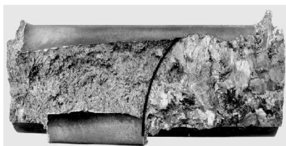
Figure 5: Fracture Surface of the Blade
