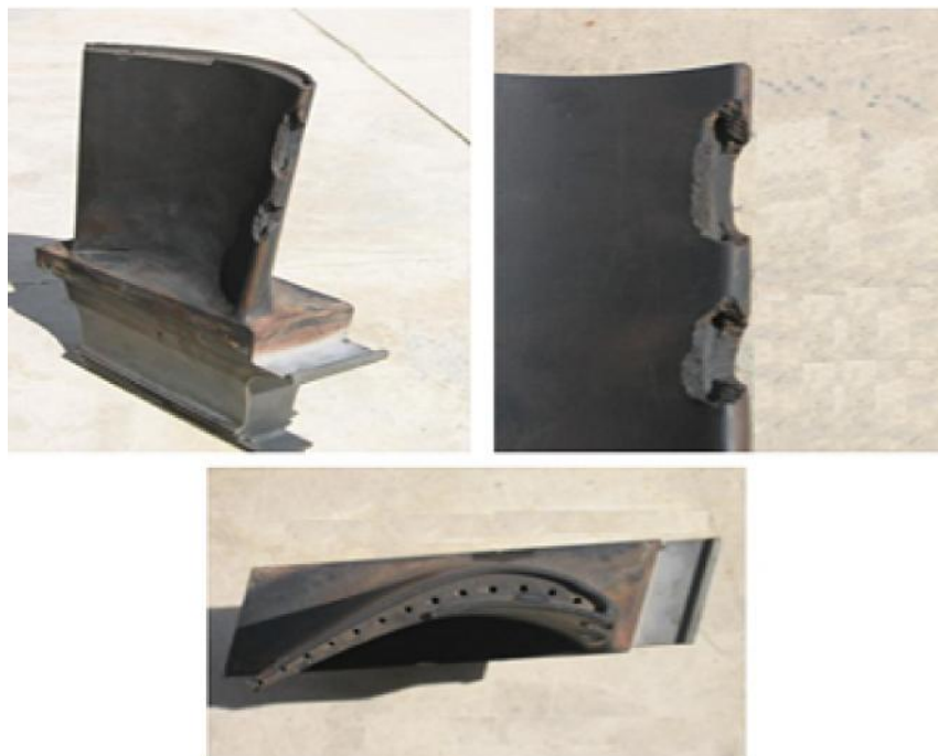
Figure 1: The General View of the First Stage Blade
