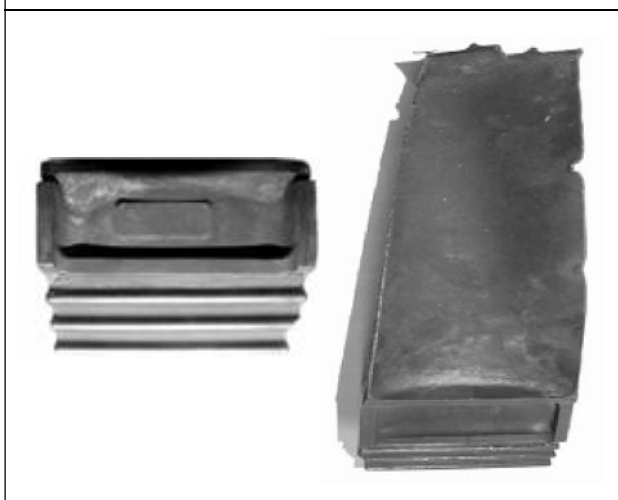
Figure 3: Blade Geometry and the Firtree Joint of a Damaged Turbine Blade
