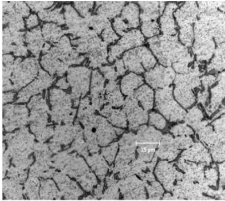
Figure 7b: Microstructure of AA-356 with 0.6 wt% of (Al-5Ti-1B) with 28 KHz Vibration (100 X)
