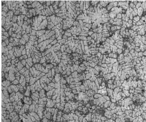
Figure 4b: Microstructure Without Grain Refiner and Without Vibration (500 X)
