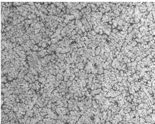
Figure 5b: Microstructure of AA-356 with 0.4 wt% of (Al-5Ti-1B) with 20 KHz Vibration (100 X)
