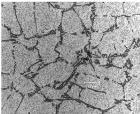
Figure 5a: Microstructure of AA-356 with 0.4 wt% of (Al-5Ti-1B) with 20 KHz Vibration (100 X)
