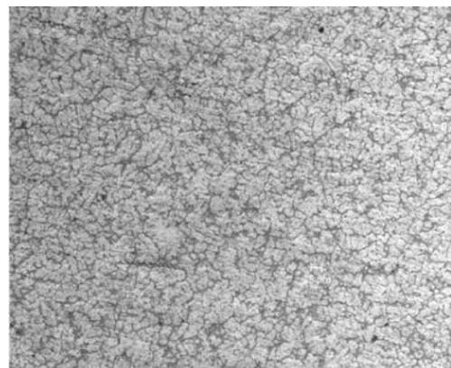
Figure 6b: Microstructure of AA-356 with 0.6 wt% of (Al-5Ti-1B) with 24 KHz Vibration (500 X)
