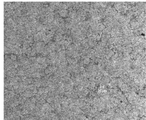
Figure 7a: Microstructure of AA-356 with 0.6 wt% of (Al-5Ti-1B) with 28 KHz Vibration (100 X)
