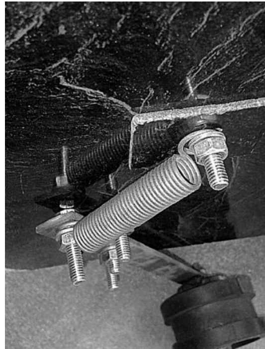
Figure 3: Showing Spring Suspension System on the Robot
