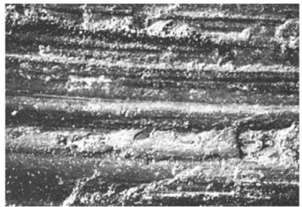
Figure 2: SEM Analysis Showing Transfer of Steel Particles to the Aluminium After Sliding
