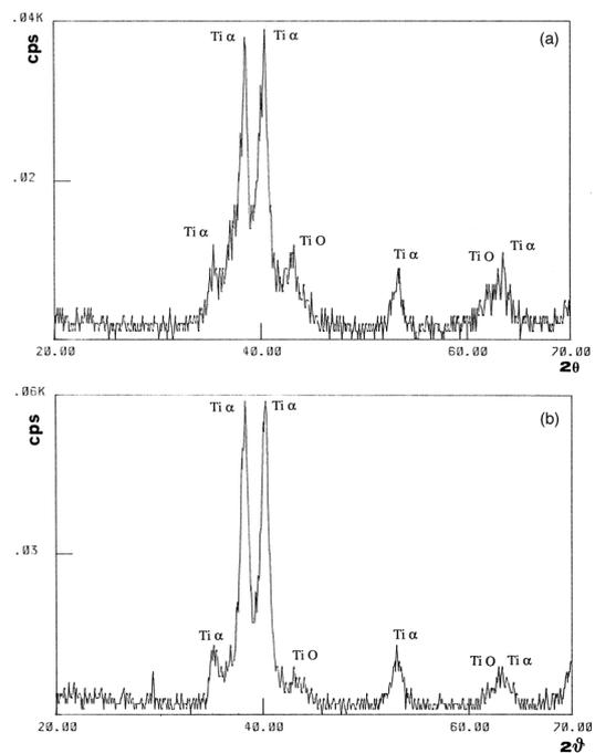
of the debris collected at the end of the tests at 0.2, 0.5 and 0.7 m/s are shown in Figure. It can be clearly noted that at the lowest sliding velocity they are constituted for the most part by a mixture of TiO and  $\alpha$ -Ti. As the sliding speed is increased the fraction of the oxides decreases and, on the other hand, the proportion of metallic  $\alpha$ -Ti constituent increases. Thus, the big plates are metallic in nature, although they may also contain some TiO compact particles.
