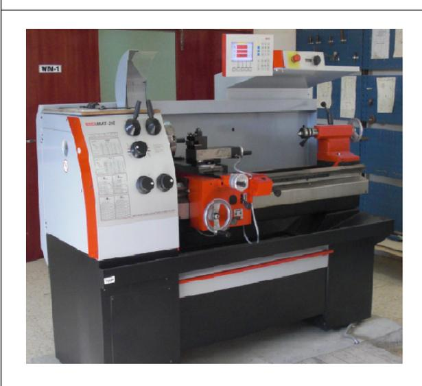
Spindle bore: 50 mm, Chuck diameter max: 200 mm.
