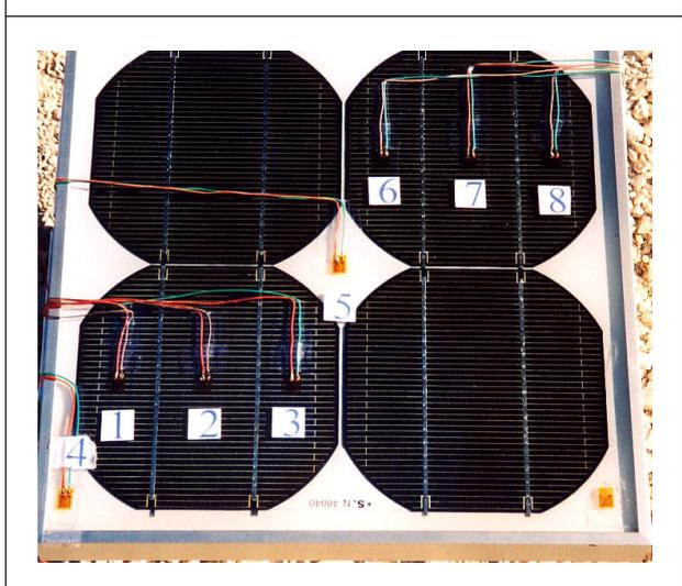
nificant zones, such as geometric centre and edges of photovoltaic cells placed in, gaps uncovered by cells, metallic conductors for electrical connections, etc. The arrangement of strain gauges on samples is shown in Figure 13.
