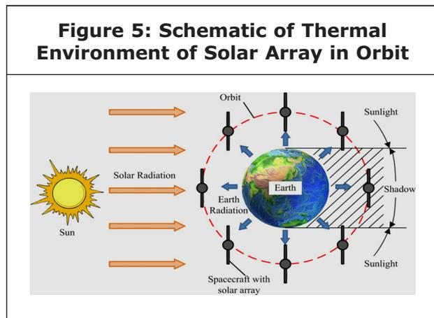
**Figure 5: Schematic of Thermal Environment of Solar Array in Orbit**
