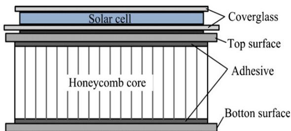
be improved in order to avoid structural damages. A careful selection and a correct assembling of materials are very important for applications of solar pane systems because the solar panel is the thing that exposed to solar radiation as shown in Figure 3.
