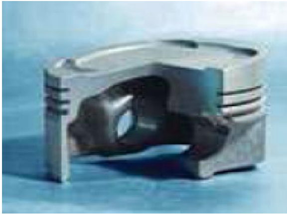
Figure 3: Piston Cast Solid Skirt Piston
