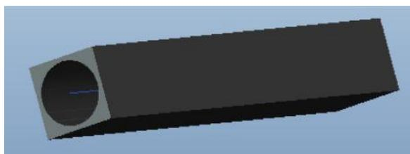
loss) and the other two sides are considered as symmetry boundary condition.
