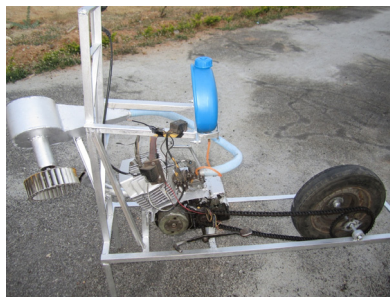
Figure 2: Fabricated Turbocharger With Engine Arrangement
