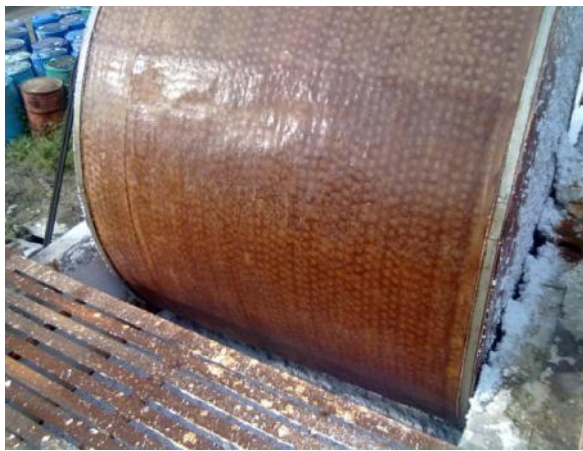
Figure 5: Single Pulp Wash Roller in Industry
