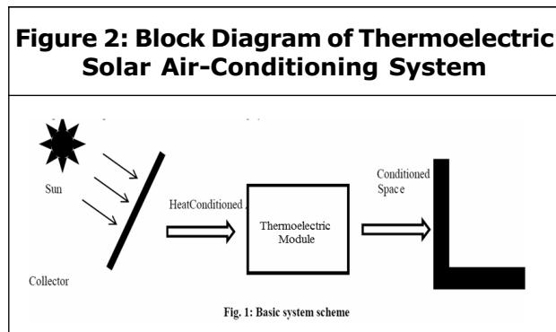
The above figure shows the basic layout of thermoelectric solar air conditioning system. Sun rays falls on solar collector which eventually converts the solar energy into electricity. That electric current is given to thermo electric module and the temperature difference occurs at two junctions. The heat is extracted from the cold junction by blowers and is given to the conditioned space.
