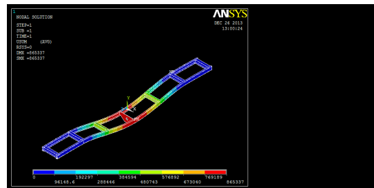
Figure 10: With Stiffener - Displacement Vector Sum
