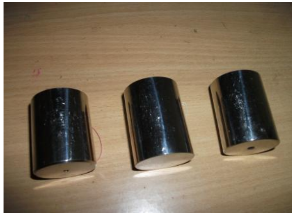
Figure 1: AISI 316 Austenitic Stainless Steel Rods
