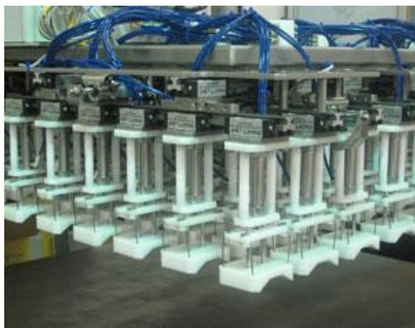
Figure 8: Specialized Needle Grippers are Used in Depanning Muffins and Other Baked Goods (Courtesy of SAS Automation LLC)
