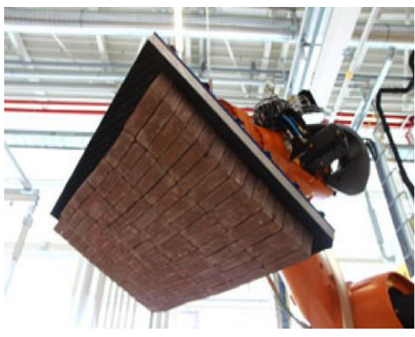
Figure 3: Large, Engineered-Foam Vacuum Gripping System Hangs Brick Pavers with Ease (Courtesy of Schmalz Inc.)
