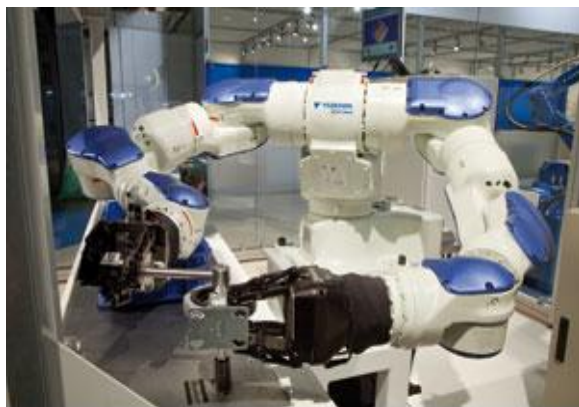
Figure 6: A Dual-Arm Robot Equipped with 3-Finger, Anthropomorphic Grippers Performs an Assembly Task (Courtesy of Robotiq)
