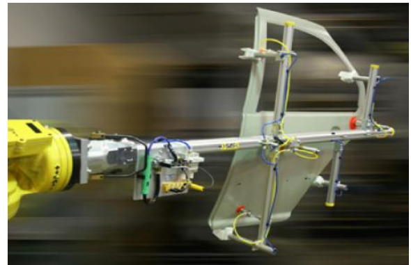
Figure 4: Hybrid End Effector Developed by SAS Automation
