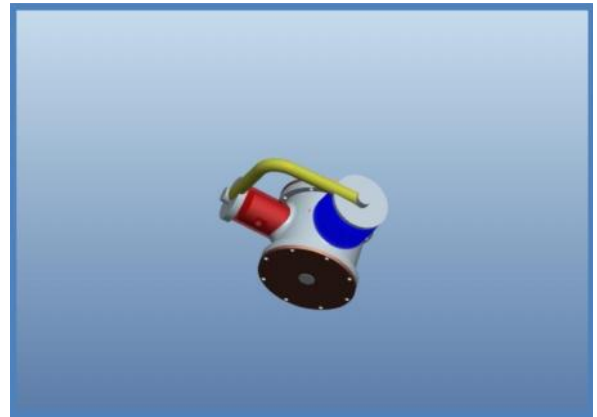
Figure 5: A Pro-e Model of an Alpha Stirling Engine
