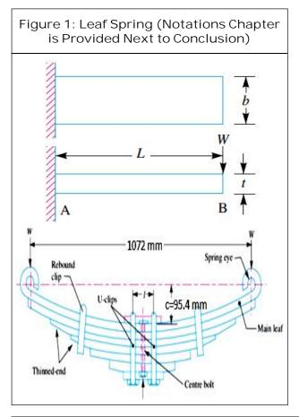
Since analyzing half of the leaf spring is enough, half of the applied force would have been taken. But here we took as it is to account over loadings of the vehicle and flexures of the leaf spring.
