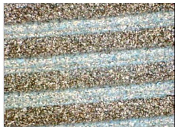
Figure 2: PLate Texture by Microgrooving (Facing) at 50X
