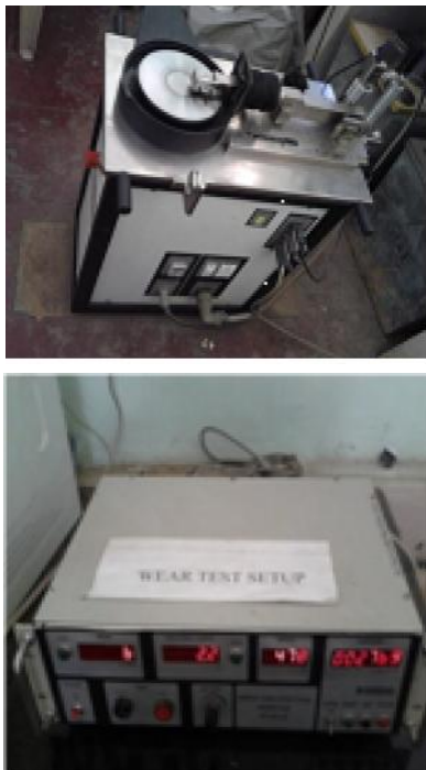
Figure 1: Set Up to Perform an Abrasive Wear Test on Pin-on-Disc
