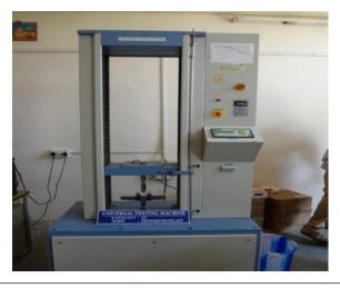
specimens are supported as a simple beam, with the compressive load applied at midpoint, and maximum fiber stress and strain calculated. The three point bending flexural test measures bend or fracture strength, yield strength, modulus of elasticity in bending, flexural stress, flexural strain, and flexural stress strain materials response. Flexural strength represents the highest stress experienced within the material at its moment of rupture.
