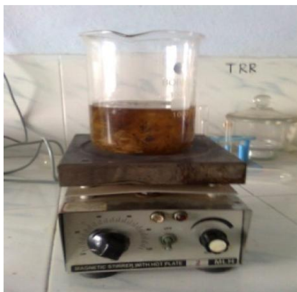
Figure 3: Heating and Stirring of Fibres
