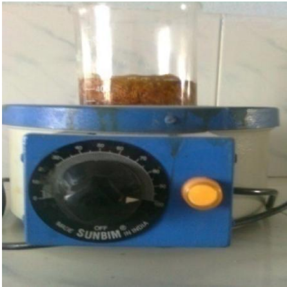
Figure 4: Treating of Fibre with \text{HNO}_3
