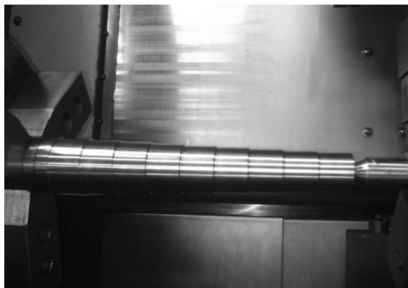
Figure 1: Experimental Setup for Turning a Nine Stepped Cylindrical Work Piece of EN8 Material on CNC Lathe Machine
