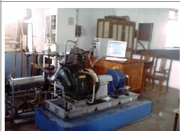
Figure 3: Experimental Set Up for an Insulated Diesel Engine
