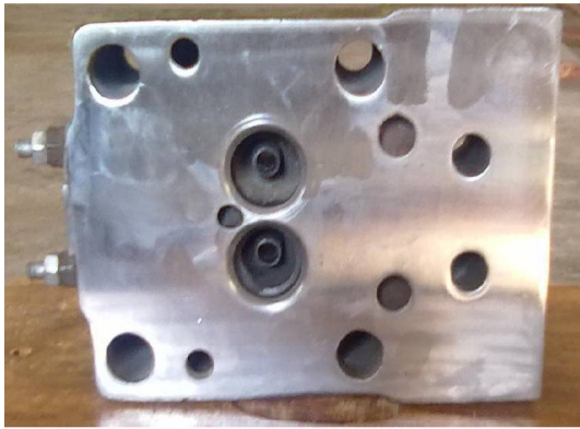
Figure 2: PSZ Coated Cylinder Head
