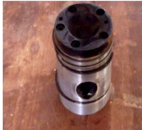
Figure 1: Aluminum Crown with an Air-Gap Insulation
