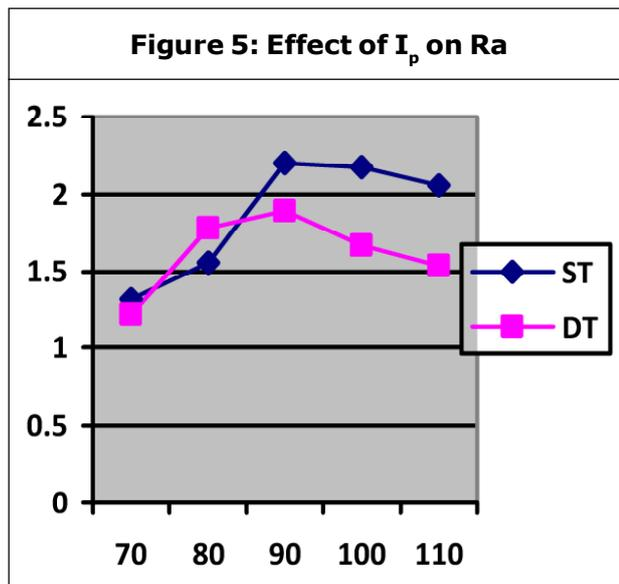
The graph shows that the roughness first slightly increases and then decreases with increase in peak current. However the increase in roughness due to increase in peak current in case of double tempered test piece is less than that of single tempered test piece and the pattern of variation in roughness is near about same in case of both the type of test pieces.
