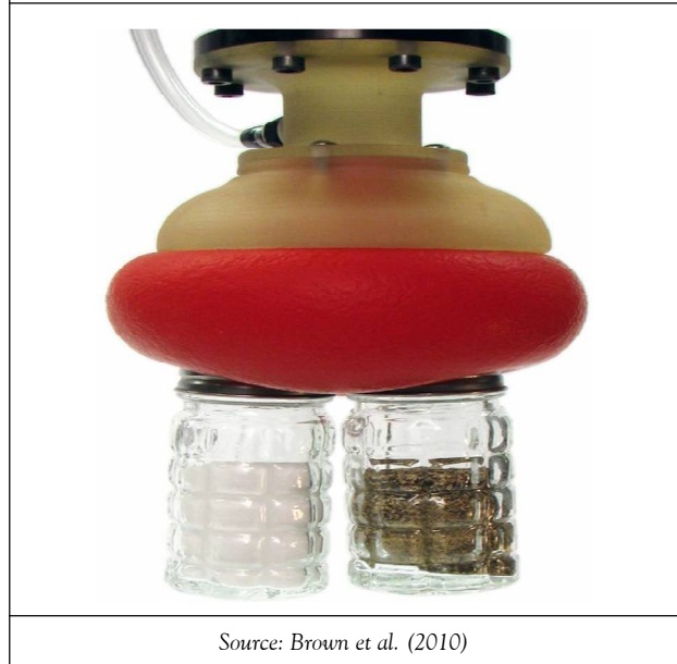
Figure 11: A Universal Gripper is Able to Grip a Wide Variety of Objects Without Grasp Planning or Sensory Feedback. Multiple Objects Can Be Gripped at Once
