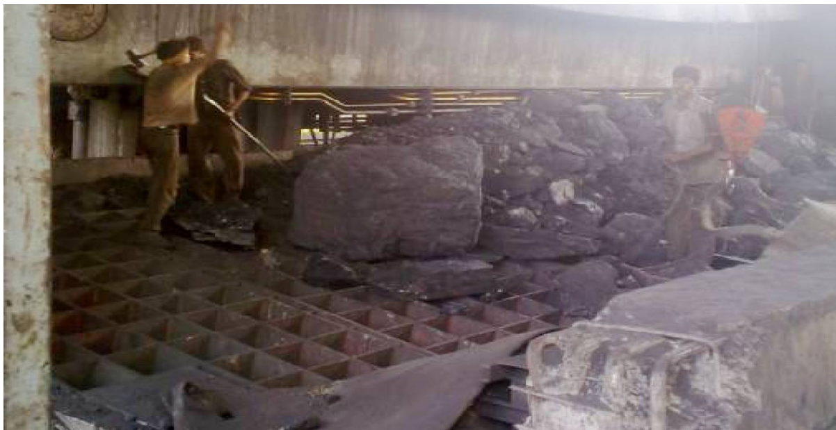
Figure 2: Iron-Gird with Large Lump Size of Coal
