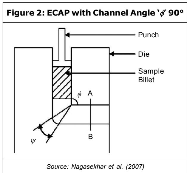
to all other channel angle while keeping the outer corner angle as  $10^\circ$  (Nagasekhar *et al.*, 2007). Figure 2 illustrates the above condition.
