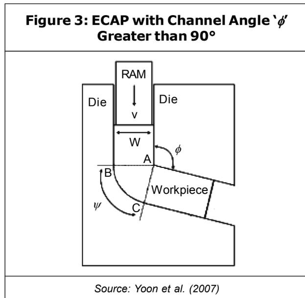
The less sheared zones are formed in non-strain hardening materials of the round corner die conditions and in strain hardening materials. In the strain hardening materials,
