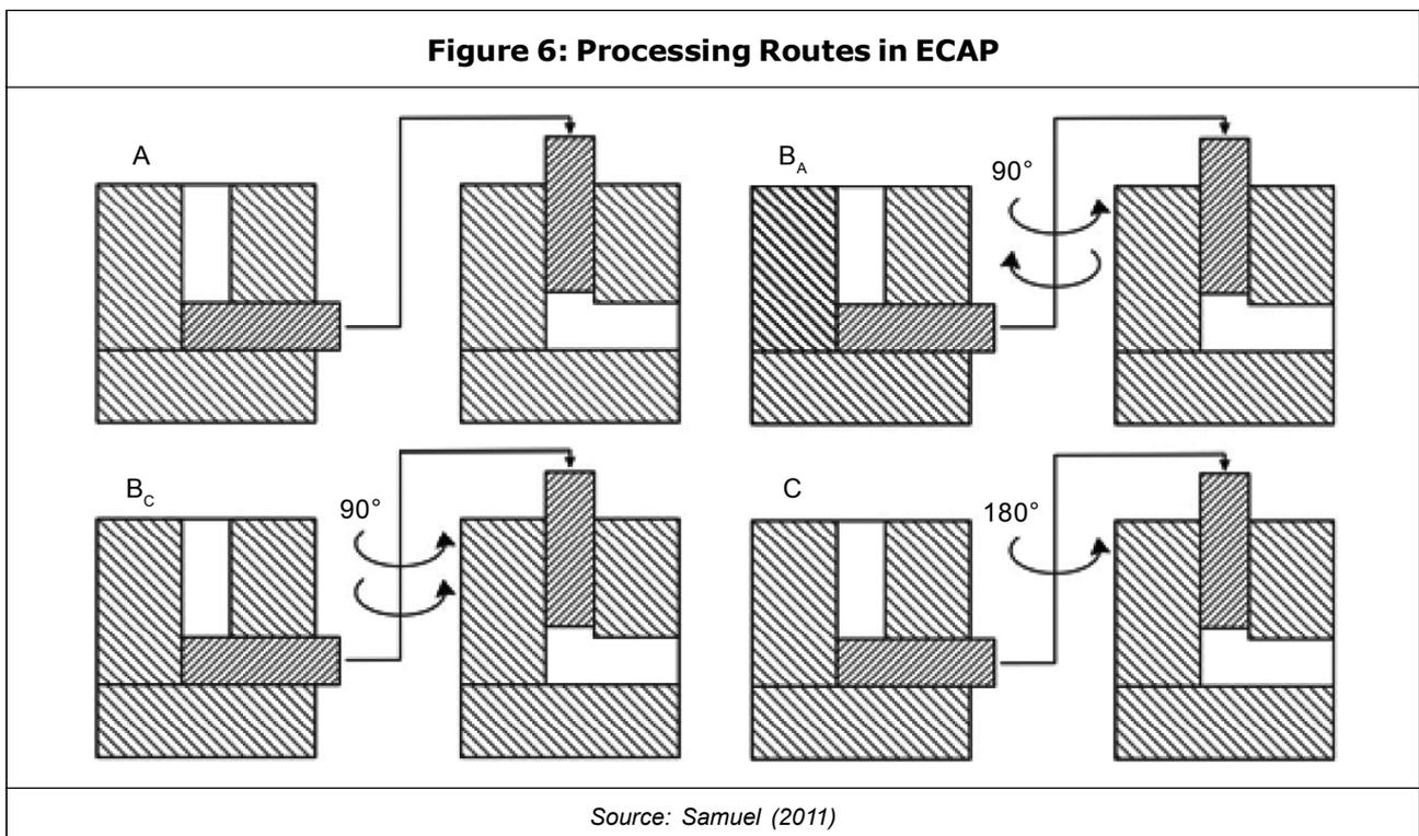
For Al6082 alloy processed through route C, The dislocation density and the subgrain size reached their maximum and minimum values, respectively, even after 1 pass. The yield strength increased monotonously even after the saturation of the dislocation density and the grain size indicating that the more equilibrated high angle grain boundaries have higher strengthening effect than the non-equilibrium boundary structures (Sandip *et al.*, 2008).
