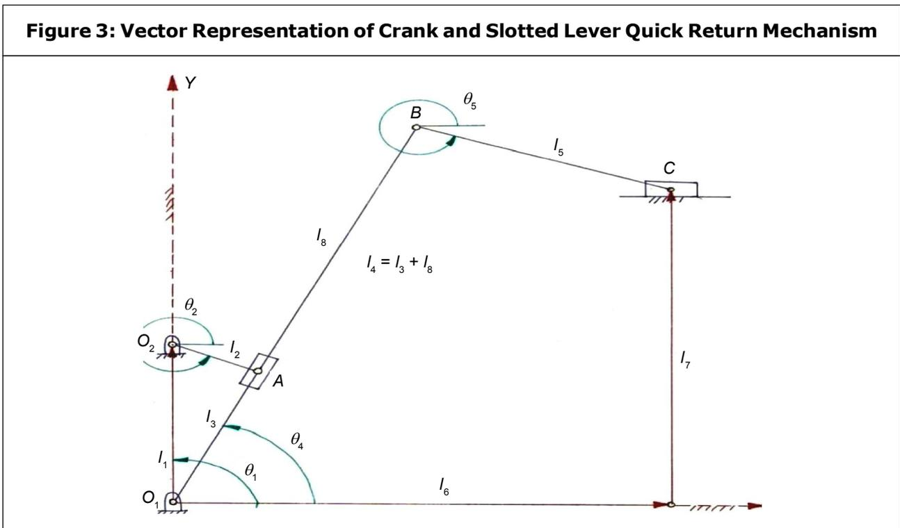
these two loops, the following sections will go through the kinematic analysis of the Crank and slotted lever Quick Return Mechanism.
