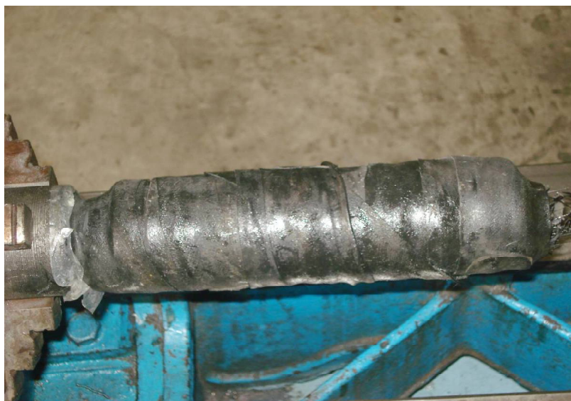
Figure 3: Shrink Tape Wound on Mandrel
