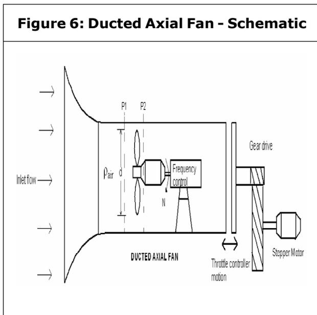
The flow enters the test duct through a bell mouth entry of cubic profile. The bell mouth performs two functions: it provides a smooth undisturbed flow into the duct and also serves the purpose of metering the flow rate.
