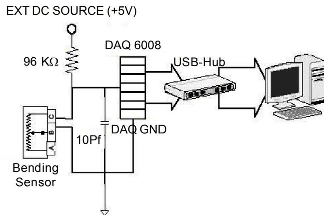
A far better solution is to provide the operator with a single manual control for all the joints angle of the robot hand, and to rely on a control system to process the input angles and produce the high-level task applied to the tele-operated robot hand. In OCU-Hand, we have applied a single bending sensor to read the angle of each finger of the operator and developed a unique
