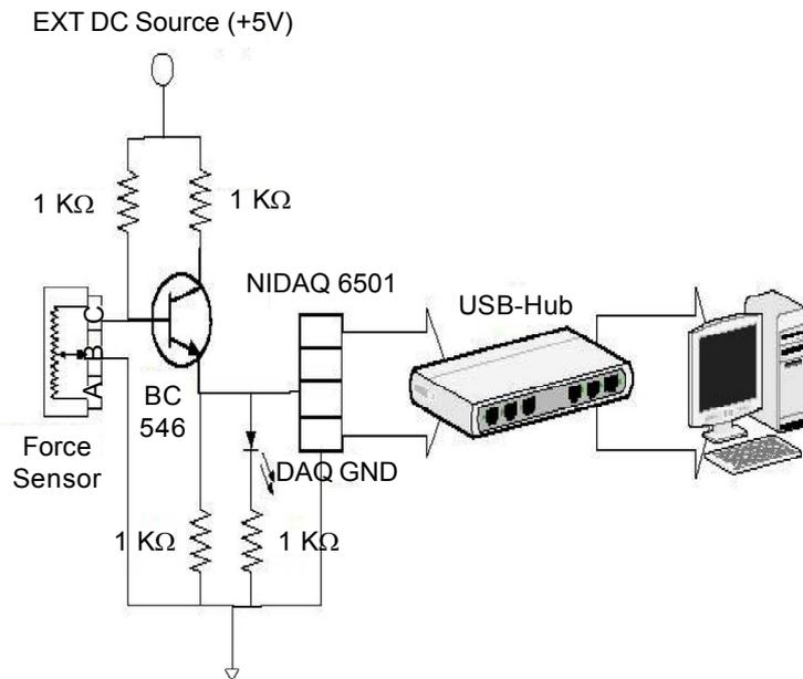
**Figure 8: Light-Weight Tele-Operating Glove and Interface**
