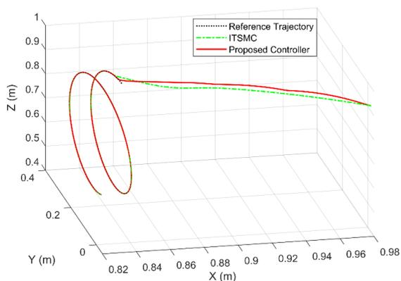
Figure 2. Required route and actual route under ITSMC and PP-ITSMC
