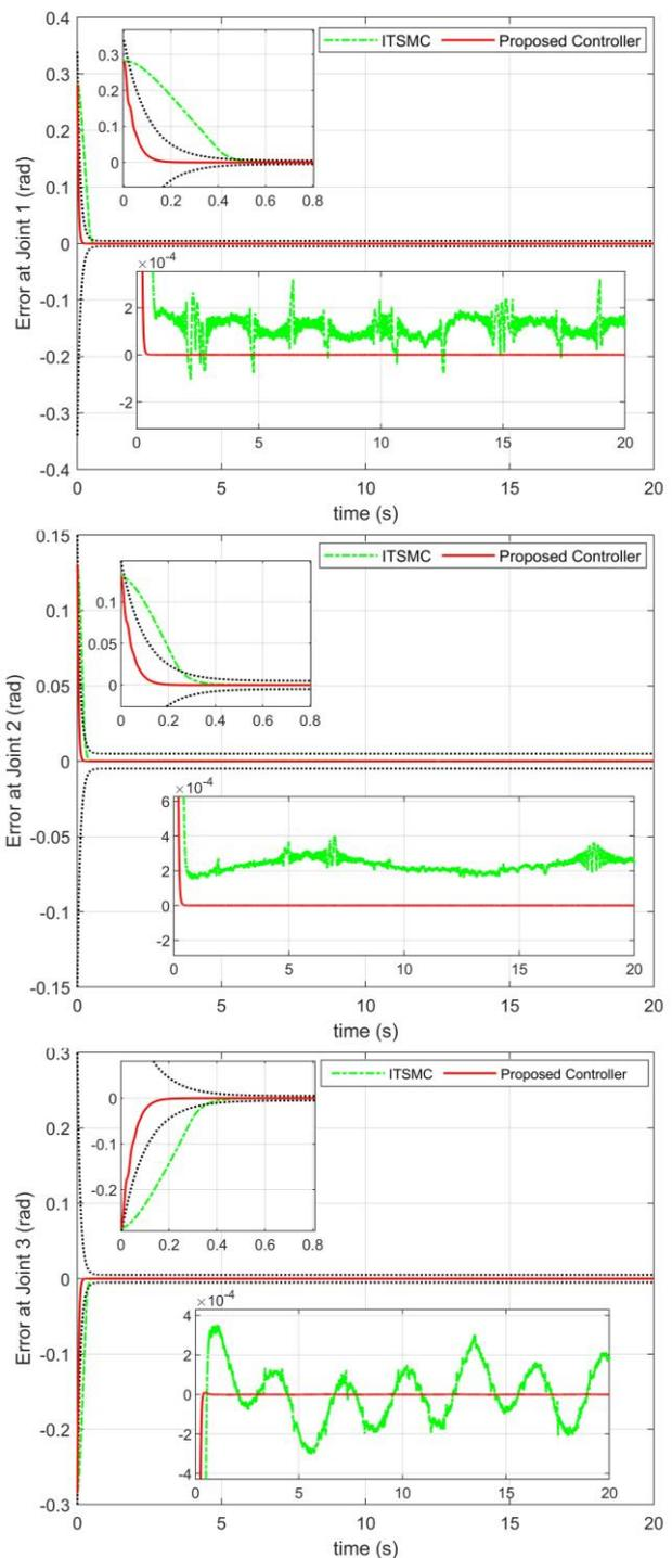
Figure 3. Time histories of the tracking errors at each Joint
