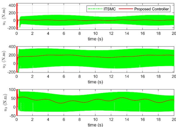
Figure 6. Control Torques of the ITSMC and the PP-ITSMC.
