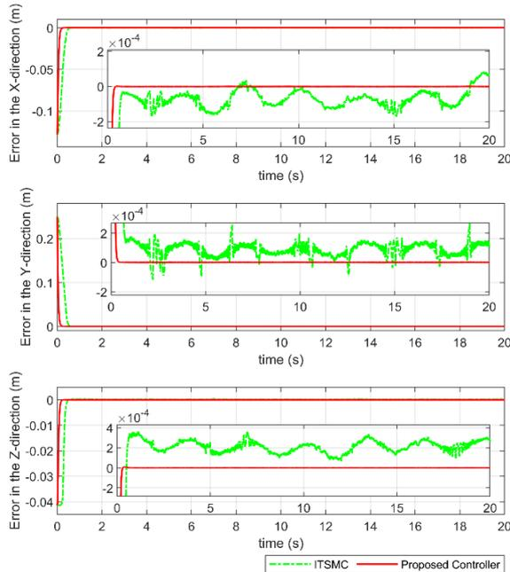
Figure 4. Time histories of X-axis errors, Y-axis errors, and Z-axis errors.
