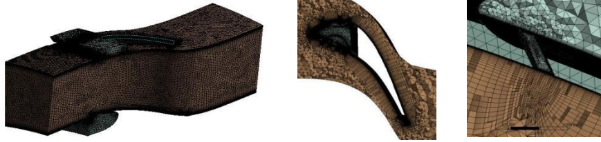
Figure 3. Basic grid model appearance of the Kuznetsov NB with internal cavity at the leading edge.
