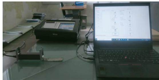
Figure 2. Roughness test process with surfest SJ 310 Mitutoyo
