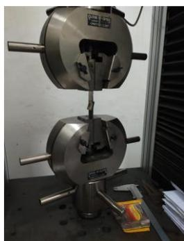
Figure 4. Tensile test machine
