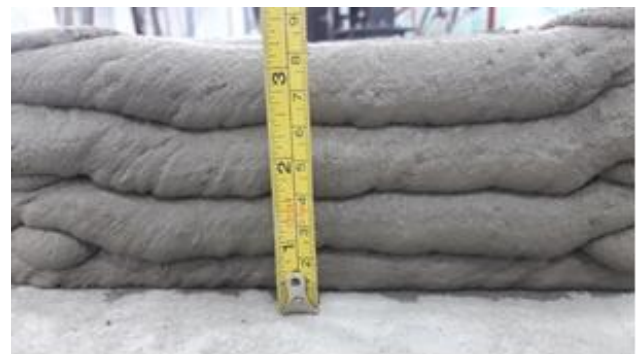
Figure 8. Deformation of the printed layer without gypsum powder.
