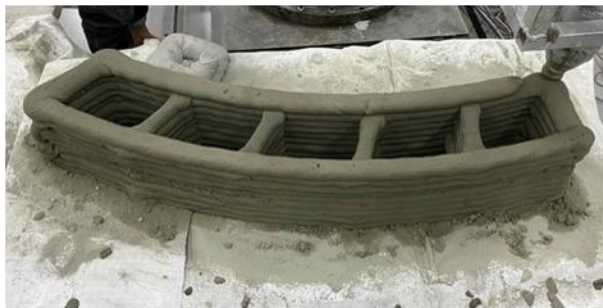
Figure 4. Actual wall structure after completion by concrete 3D printing.
