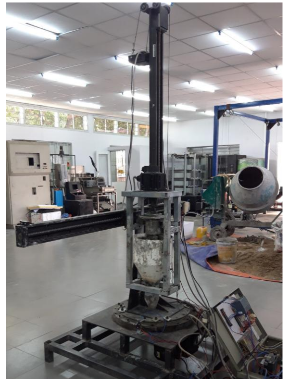
Figure 2. Manipulator and extruder used for research.
