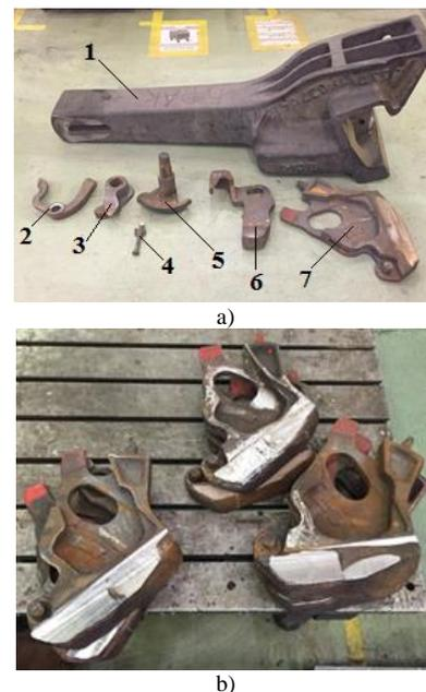
Figure 1. Body and parts of the coupling device: a - automatic coupler housing and detailing; b - parts prepared for surfacing; 1 - automatic coupler housing; 2 - safety; 3 - lifter; 4 - bolt with lock washers; 5 - shaft lifter; 6 - locking mechanism; 7 - lock.
