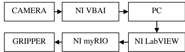
Figure 1. Block diagram of system control on the gripper.
