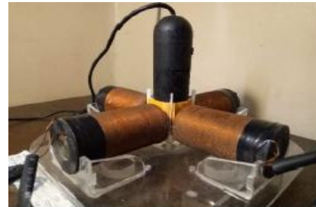
Figure 6. The adaptive suggested system for micro-particle controlling the in a 2D space [3].
