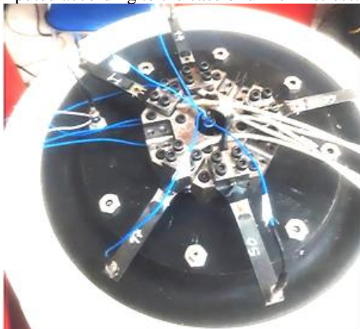
Figure 3. Specimens with strain gauges on vibrating table of LDS dynamic shaker.
