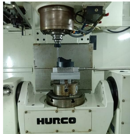
Figure 1. Installation of work pieces and force-measuring tools in the machining process
