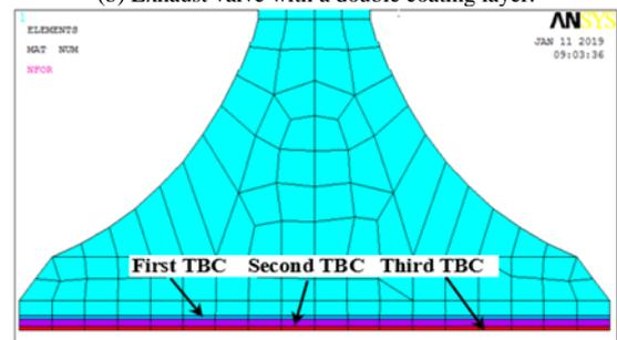
(c) Exhaust valve with a triple coating layer.
