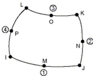
Figure 3. PLANE77 element - PLANE183 element model [22].
