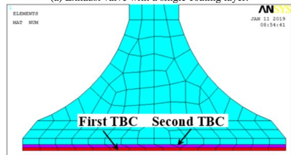
(b) Exhaust valve with a double coating layer.
