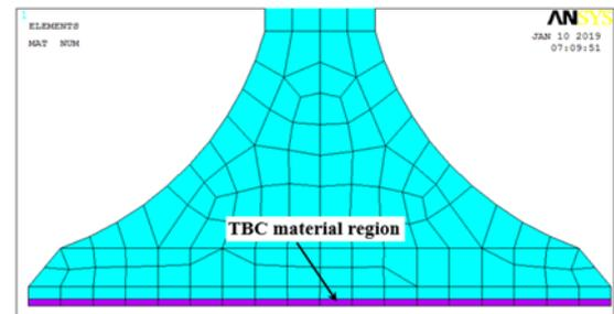
(a) Exhaust valve with a single coating layer.
