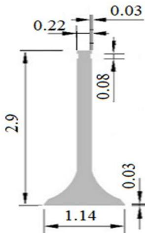
Figure 1. Exhaust valve dimensions.
