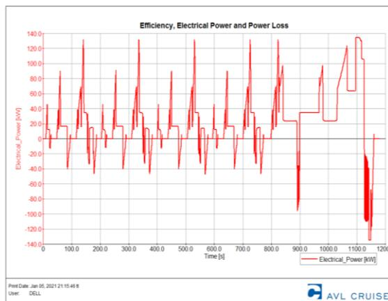
Figure 8. Electric power in NEDC cycle
