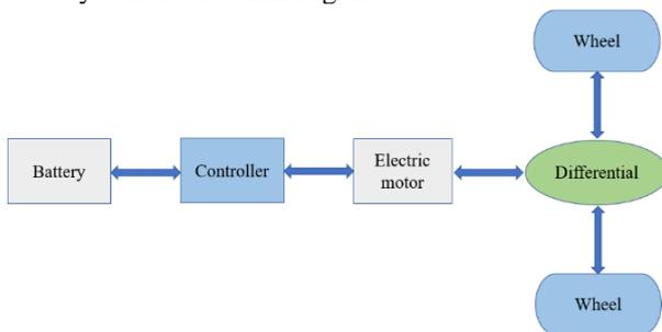
Figure 2. Electric vehicle configuration
