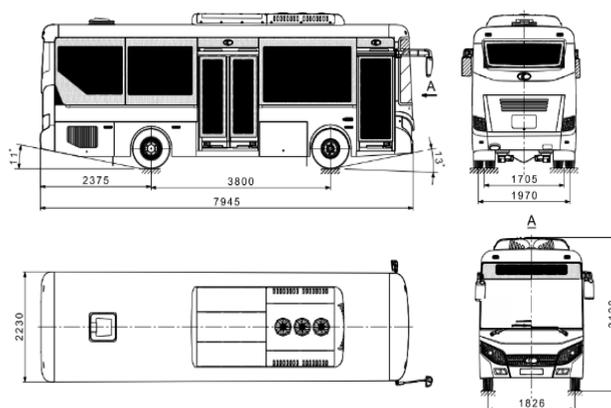
Figure 1. Vehicle overall dimension
