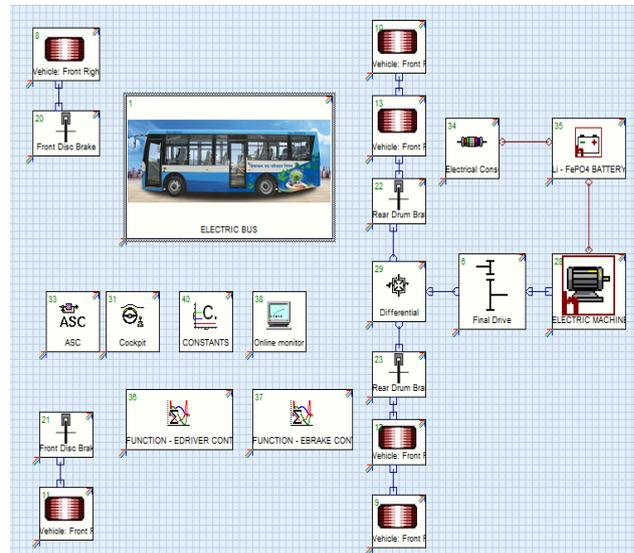
Figure 5. Model of electric vehicle in AVL CRUISE
