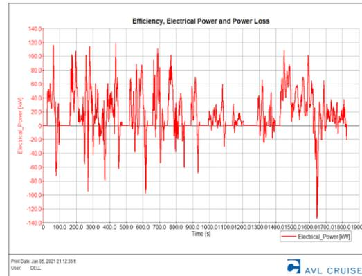
Figure 9. Electric power in Japan mode 1 Urban cycle
