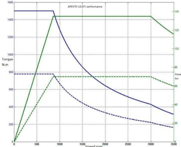
Figure 4. Drive motor characteristics of the electric vehicle
