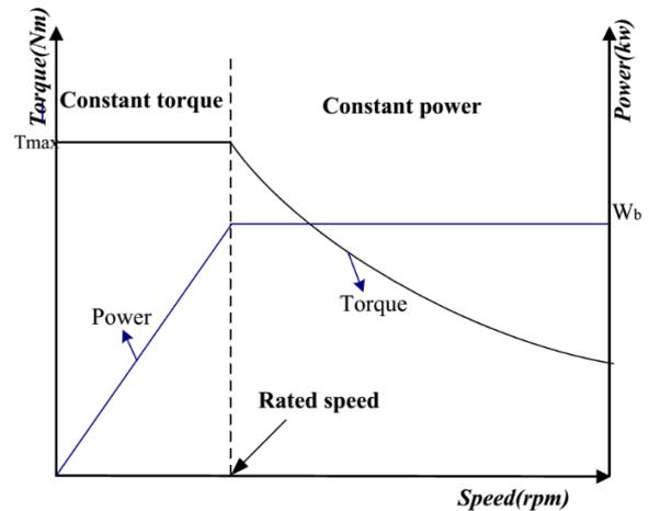
Figure 3. Electric motor characteristics
