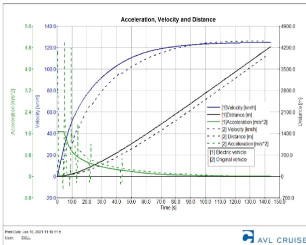
Figure 12. Driving performance from standstill to maximum velocity
