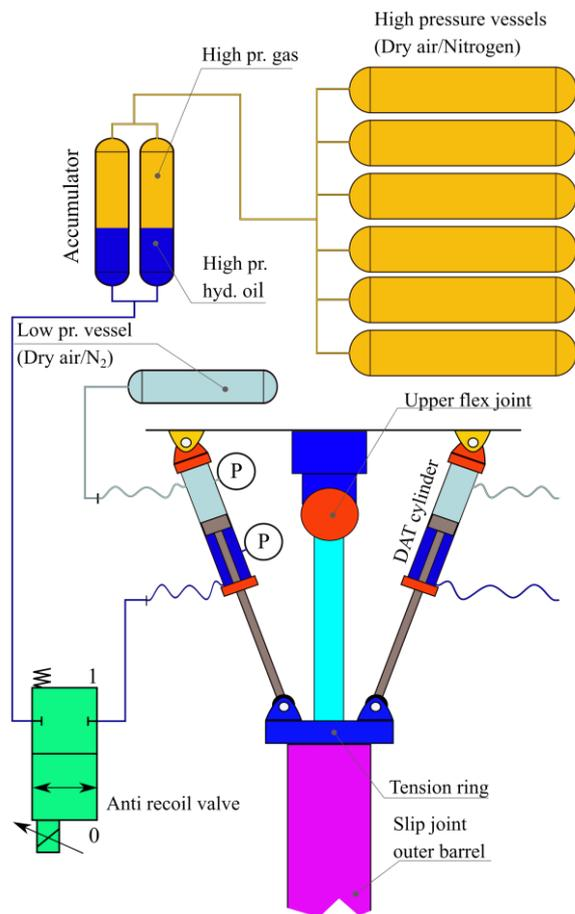
Figure 2. The hydropneumatic circuit.
