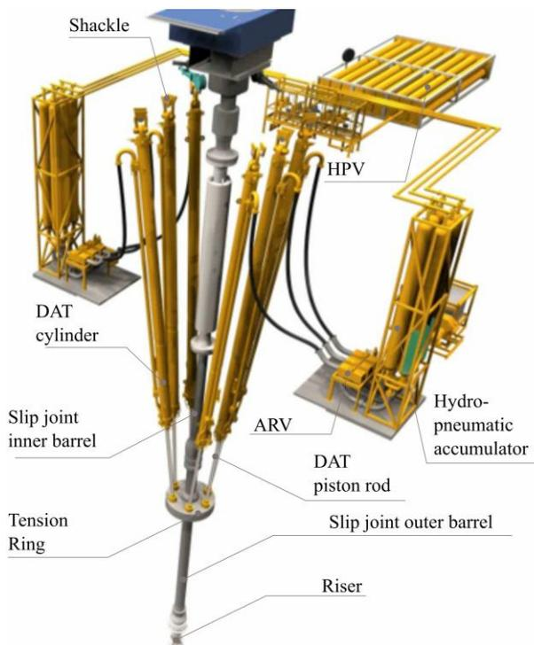
Figure 3. DAT system arrangement (courtesy NOV).
