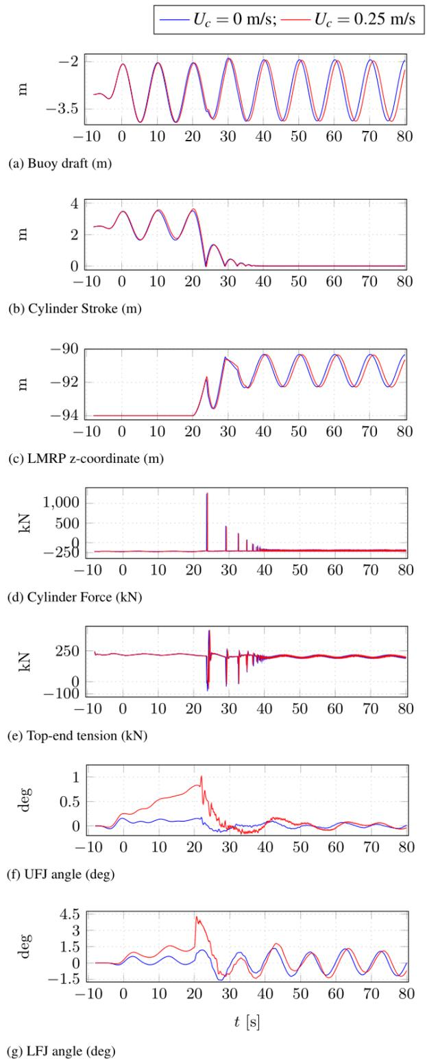
Figure 8. Basic realistic system response to disconnect in waves of height 2 m and different conditions of current.
