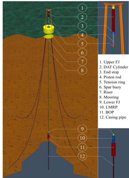
Figure 4. Concept of the basic realistic riser tensioner system.
