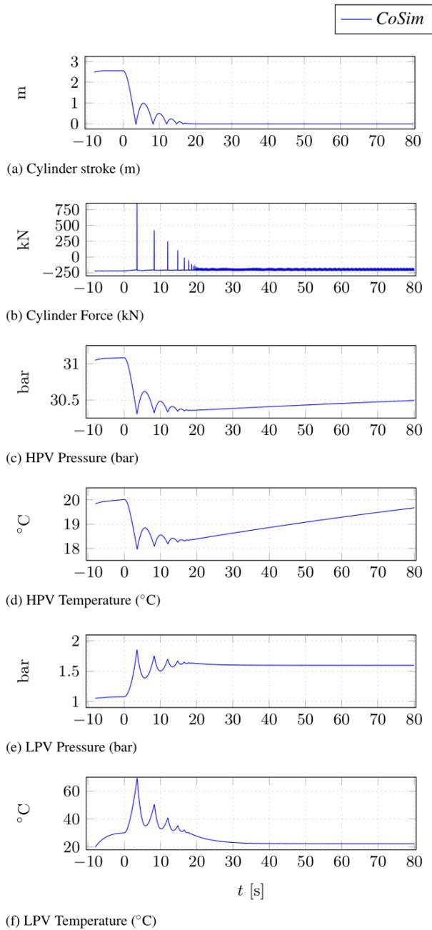
Figure 7. Basic realistic system response to calm water disconnect (SimulationX results).
