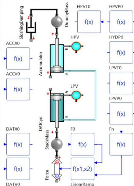
Figure 5. SimulationX component model of the hydro-pneumatic tensioner.
