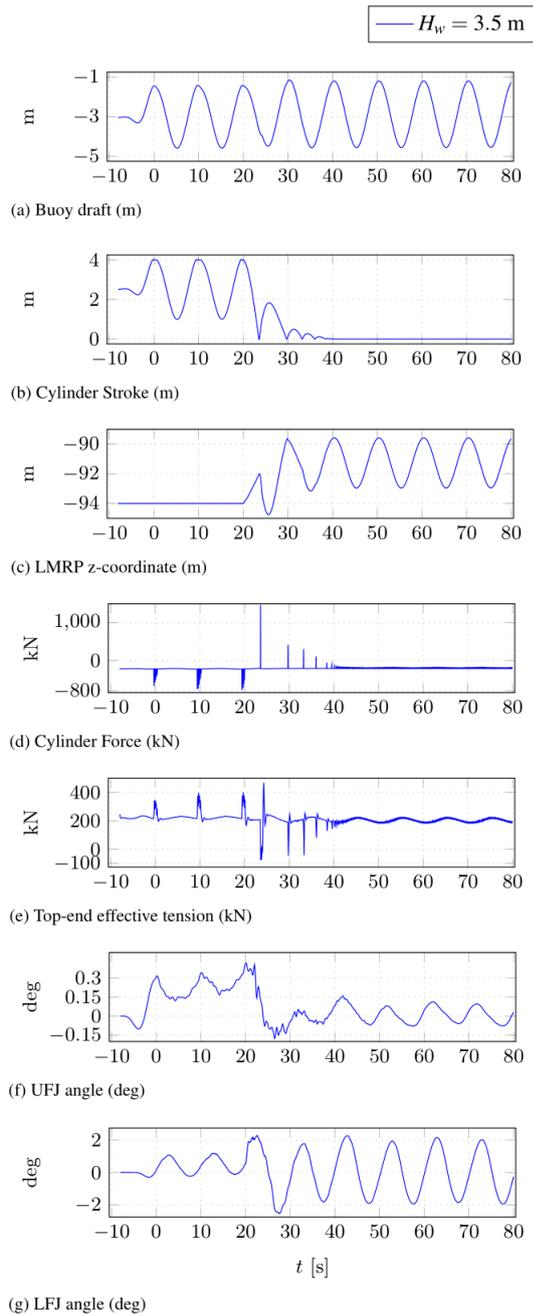
Figure 9. Basic realistic system response to disconnect with piston hitting gland-end while in compensation mode.
