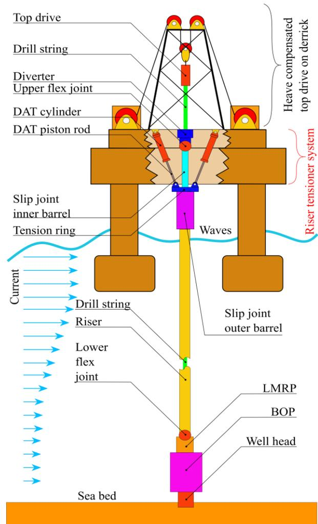
Figure 1. General arrangement of the riser tensioner system (DAT).
