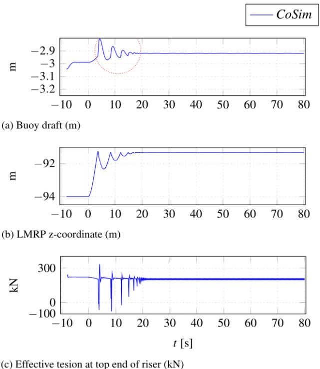
Figure 6. Basic realistic system response to calm water disconnect (*OrcaFlex* results).
