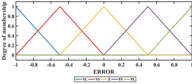
Figure 7. Membership functions for fuzzy input variables (error)
