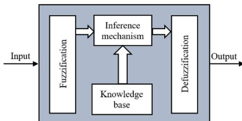
Figure 2. The FLC block diagram
