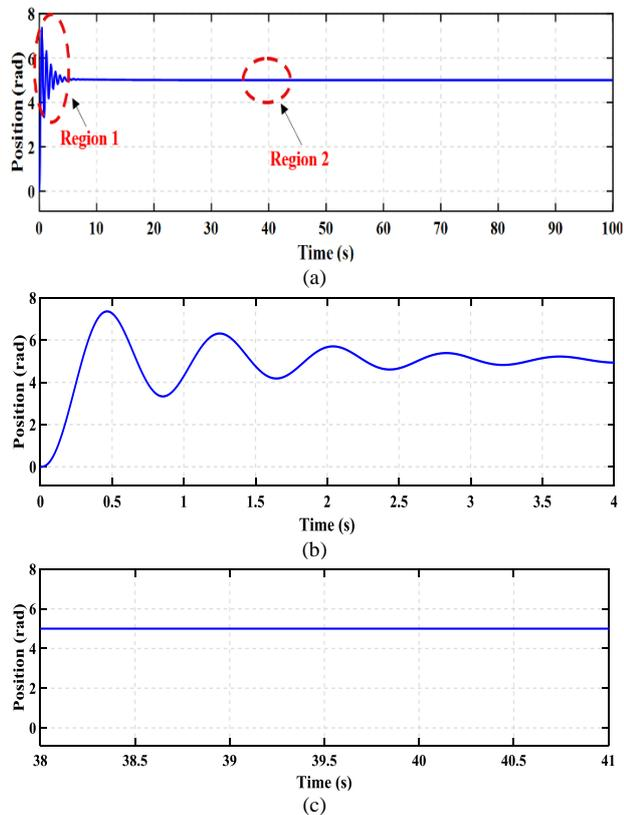
Figure 4. System step reference: (a) System step reference based on FLC (b) Close view of Region 1 (c) Close view of Region 2
