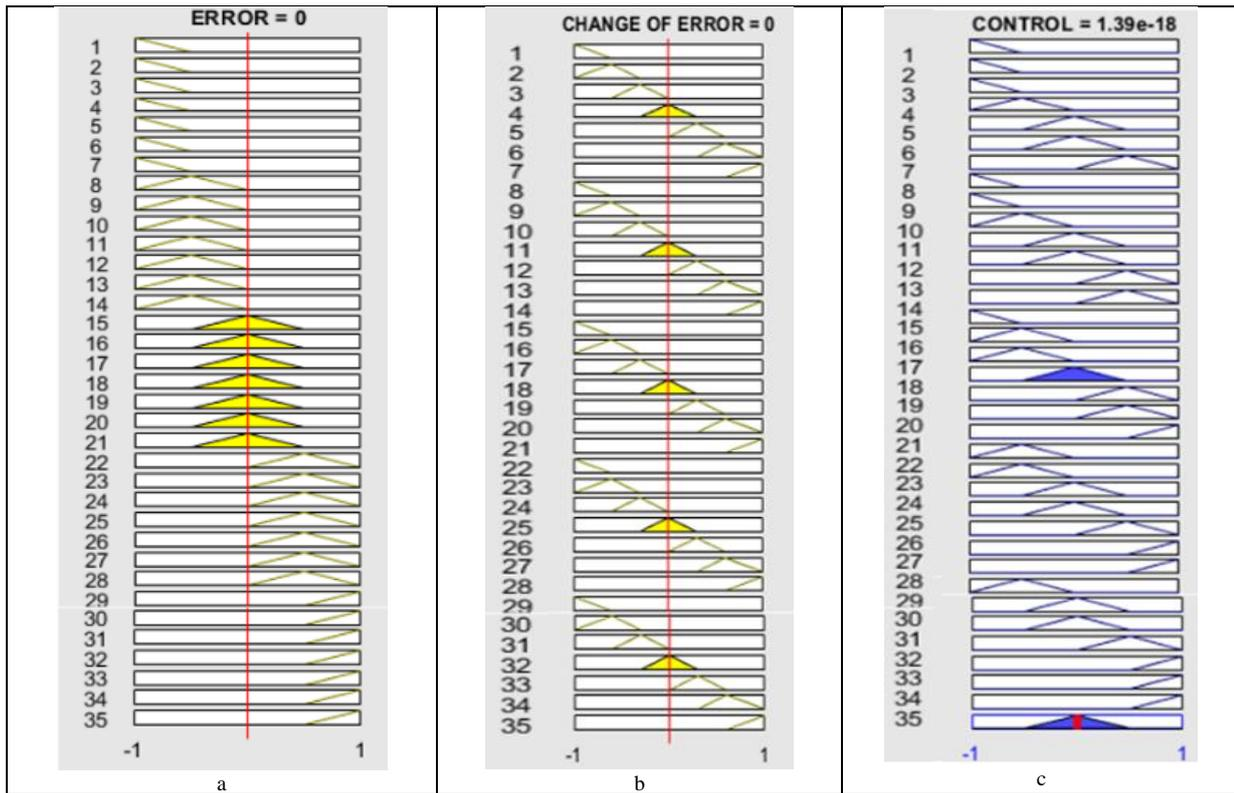
Figure 12. Rule viewer FLC: (a) Error (b) Change of error (c) Control
