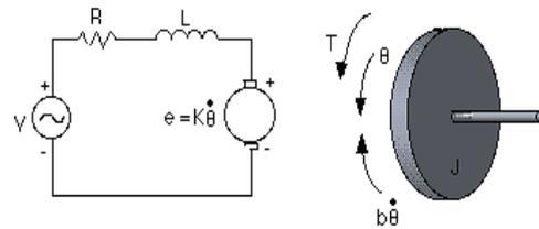
Figure 1. Separately excited D.C. motor (DC motor equivalent circuit and free-body diagram of the rotor)
