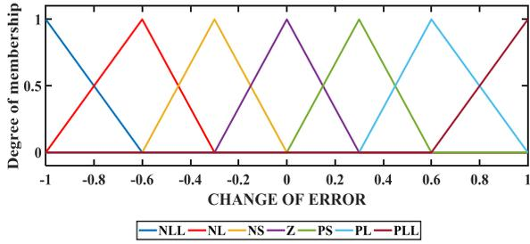
Figure 8. Membership functions for fuzzy input variables (change of error)
