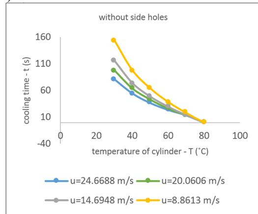
Figure 6. Relationship between temperature of cylinder and cooling time for cylindrical sample No.1 at different air velocities.
