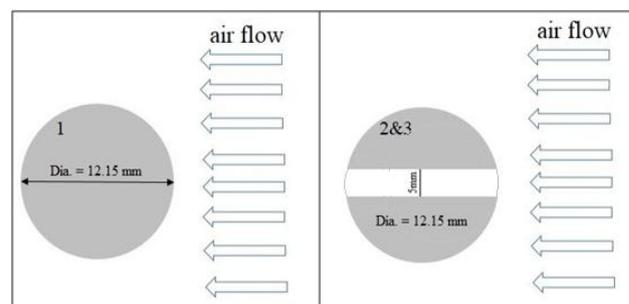
Figure 4. Direction of air flow with cylinder (cross-flow).
