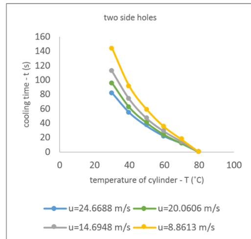
Figure 7. Relationship between temperature of cylinder and cooling time for cylindrical sample No. 2 at different air velocities.
