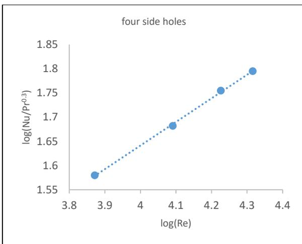
Figure 19. The empirical relationship between the (Log Re) and (Log Nu/Pr<sup>0.3</sup>) for cylindrical sample No.3.
