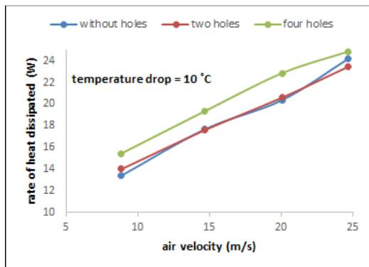
Figure 13. Relationship between air flow velocity and rate of heat dissipated for three cylinder samples.
