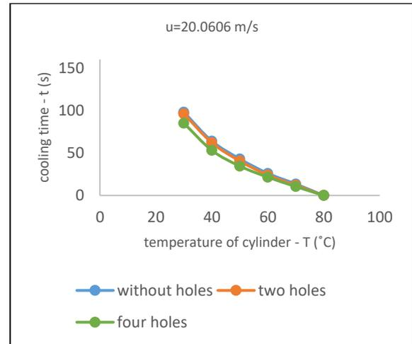
Figure 10. Relationship between temperature of cylinder and cooling time for three cylinder samples at ( $u=20.0606$  m/s).
