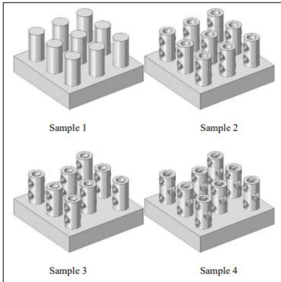
Figure 1. Four designs of pin fins as the heat sinks [18].
