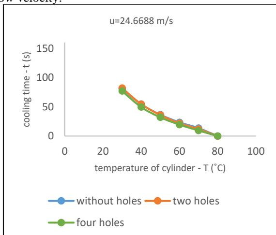
Figure 9. Relationship between temperature of cylinder and cooling time for three cylinder samples at ( $u=24.6688$  m/s).
