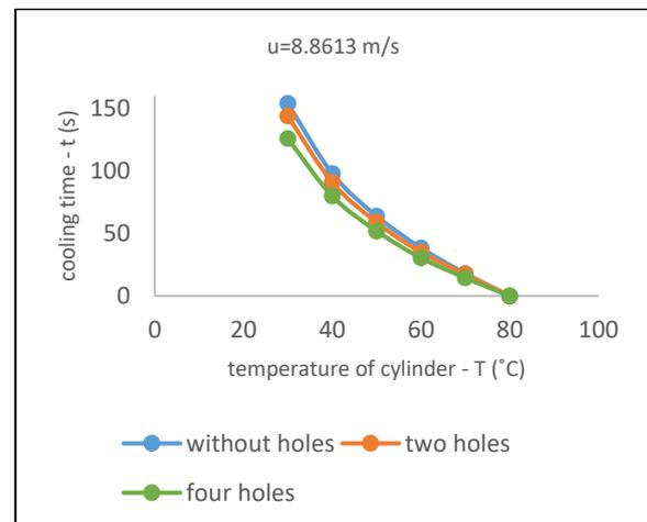
Figure 12. Relationship between temperature of cylinder and cooling time for three cylinder samples at ( $u=8.8613$  m/s).
