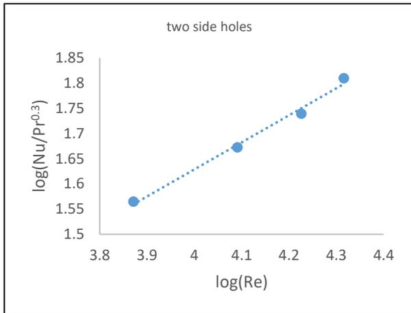
Figure 18. The empirical relationship between the (Log Re) and (Log Nu/Pr<sup>0.3</sup>) for cylindrical sample No.2.
