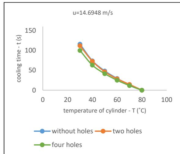
Figure 11. Relationship between temperature of cylinder and cooling time for three cylinder samples at ( $u=14.6948$  m/s).
