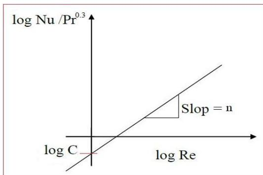
Figure 5. Empirical relation between  $(\text{Log } Re)$  &  $(\text{Log } Nu/Pr^{0.3})$ .
