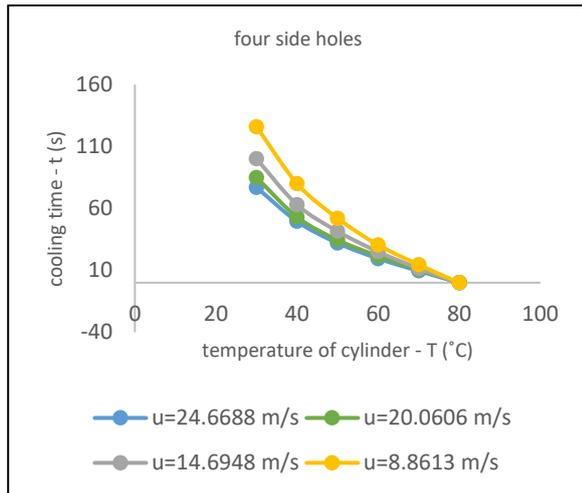
Figure 8. Relationship between temperature of cylinder and cooling time for cylindrical sample No.3 at different air velocities.
