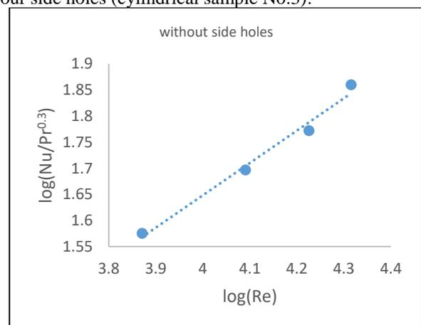
Figure 17. The empirical relationship between the (Log Re) and (Log Nu/Pr<sup>0.3</sup>) for cylindrical sample No.1.
