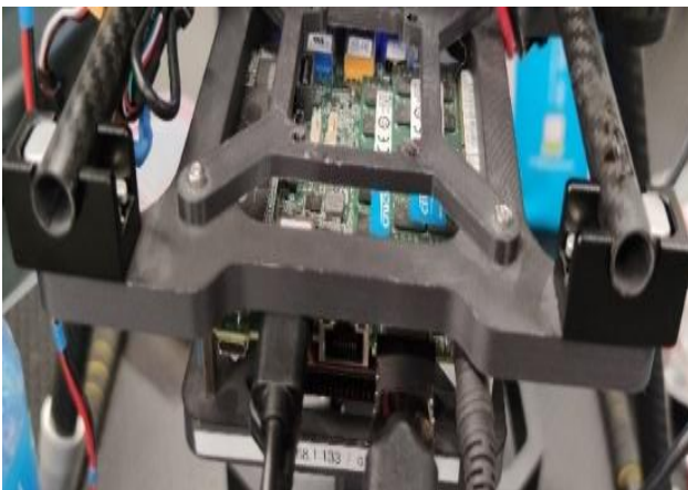
Figure 2. Intel NUC mounting assembly
